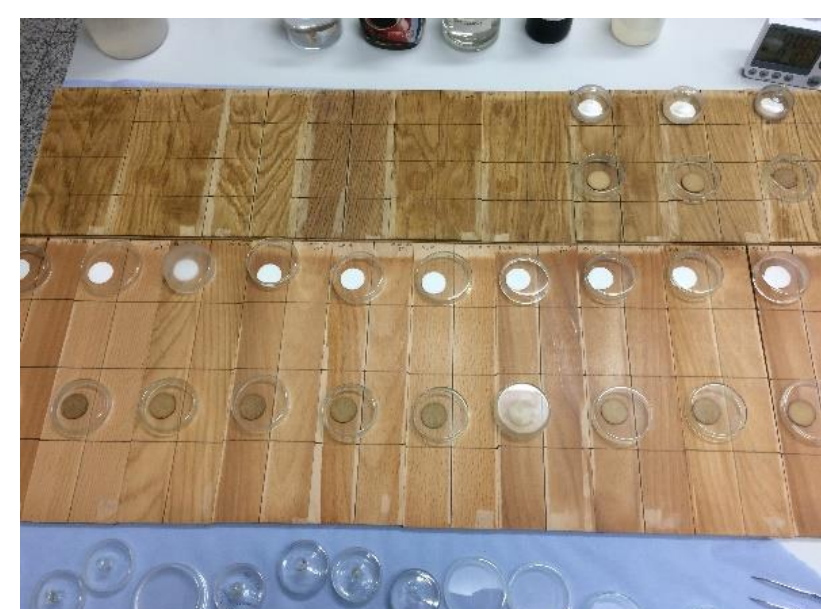
Figure 5: wood specimens with test fluids
