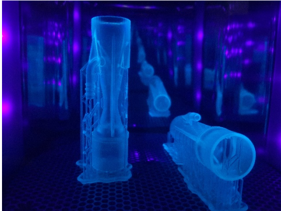
An additive manufactured valve for ventilators from the 3D printer of the DRESDEN-concept partners.
