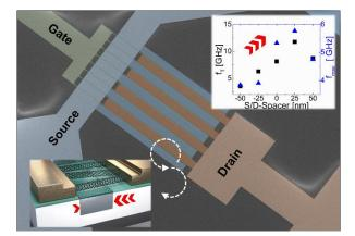
The analyses showed that an increase in transistor speed of up to 18 percent can be achieved, at the same time improving amplifier linearity. In this study, transition frequencies of up to 14 GHz were achieved. Since this technology allows for alternative component concepts, these properties are interesting for a wide range of applications in advanced electronics even today. *¬* More
