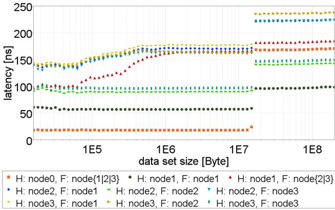
Fig. 7. Memory read latency: core in node0 accesses cache lines with *forward* copies in another node (F:) which also have different home nodes (H:). The home nodes also contain a copy which is in the *shared* state if the *forward* copy is in another node. The sharing also affects the memory latency because of stale state in the in-memory directory.
