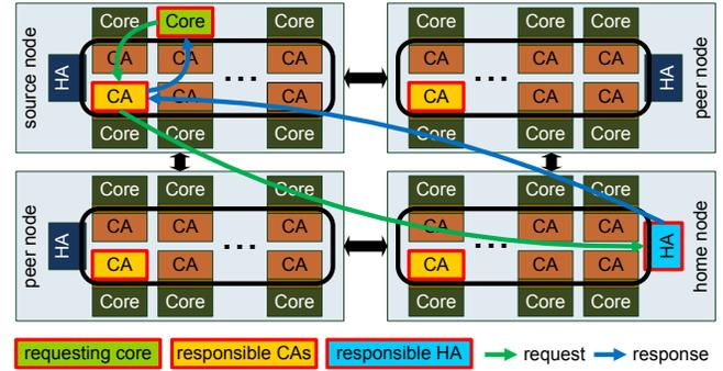
Fig. 3. The cores forward requests to the caching agents within their node. If the request cannot be serviced locally, it is forwarded to the home agent. Snoops of the CAs in the peer nodes are either handled by the CA or the HA (see Section IV-B and Section IV-C)
