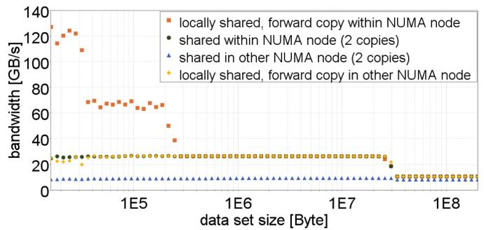
Fig. 9. Memory read bandwidth in default configuration (source snoop): Accesses to shared cache lines.
