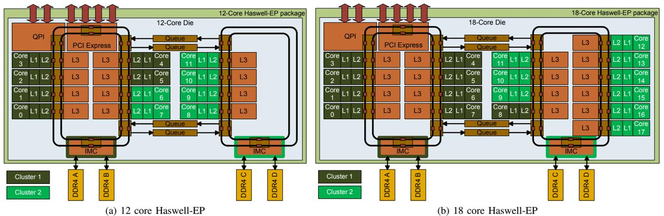
Fig. 1. Haswell-EP block diagram: There are two rings with one memory controller (IMC) each. QPI and PCIe links are connected to the first ring. The rings are connected with bi-directional queues. In the default configuration all cores can access the whole L3 cache and memory is interleaved over all four channels. The Cluster-on-Die mode splits the chip into two NUMA nodes which share one memory controller each.
