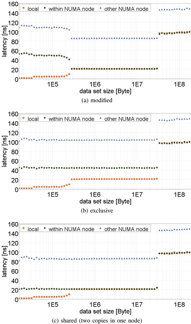
Fig. 4. Memory read latency in default configuration (source snoop): Comparison of accesses to a core's local cache hierarchy (local) with accesses to cache lines of another core in the same NUMA node (within NUMA node) as well as accesses to the second processor (other NUMA node (1 hop QPI)).
