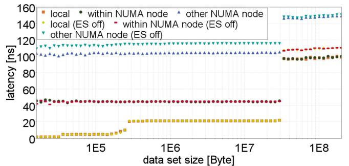
Fig. 5. Memory read latency: Comparison of source snoop and home snoop, cached data in state *exclusive*
