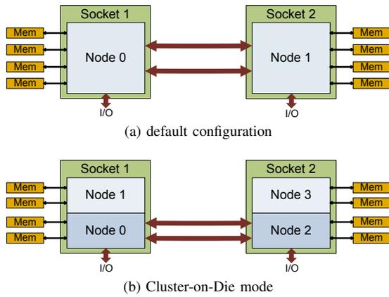
Fig. 2. Dual socket Xeon E5 v3 system: In the default configuration, the partitioned chip design is not exposed to the operating system. Therefore, the system presents itself as two NUMA nodes. If COD mode is enabled each socket is divided into two nodes, thus four NUMA nodes are visible.
