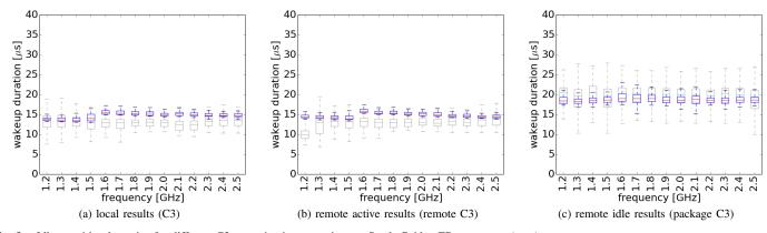
Fig. 5. Idle transition latencies for different C3 scenarios in comparison to Sandy Bridge EP processors (grey)
