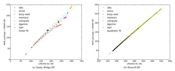
Fig. 2. Comparison of power measurements with RAPL (package + DRAM, sum of two sockets) on Sandy-Bridge EP [20] and Haswell-EP versus total system power consumption (AC) measured with a high-accuracy power meter. Note that the different x-axis ranges are due to the full speed fan settings on the Haswell-EP system which does not affect RAPL accuracy.
