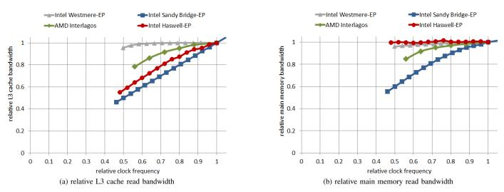
Fig. 7. Scaling of shared main memory and L3 cache bandwidth at maximum thread concurrency, normalized to the bandwidth at base frequency.
