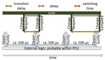
Fig. 4. Presumed mechanism for p-state changes on Intel Haswell-EP processors.
