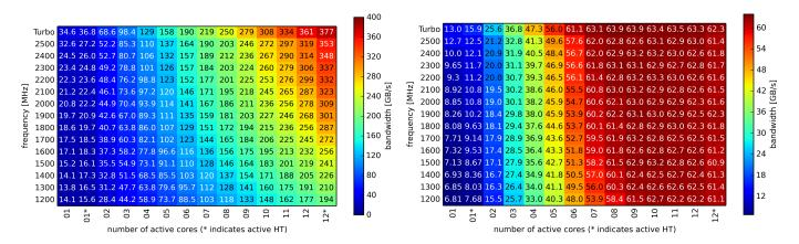
Fig. 8. Read bandwidths from Level 3 cache (left) and DRAM (right) depending on concurrency and frequency
