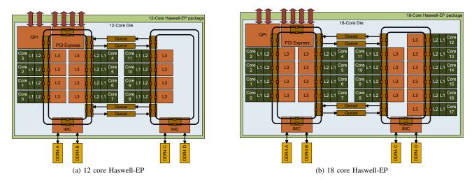
Fig. 1. Haswell-EP implementations with partitioned ring interconnect [6]. The 12-core die (left) is used for 10-core and 12-core units. The 18-core die (right) is used for 14, 16, and 18-core units.
