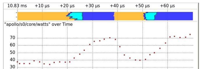
(a) 12  $\mu\text{s}$  load changes and the core power consumption (VR) on *system A*
