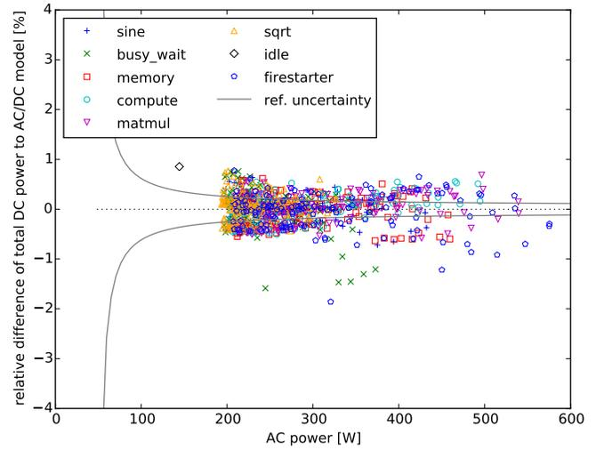
Fig. 4. Relative difference of the sum of board input Hall effect measurements compared to the quadratic PSU model of the AC reference measurement on *system A*. Includes the uncertainty bound of the reference measurement.
