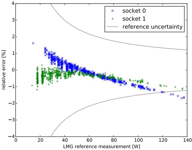
Fig. 6. Relative difference of the 12 V per-socket shunt measurements compared to 12 V per-socket reference measurements on *system B*. Includes the uncertainty bound of the reference measurements.
