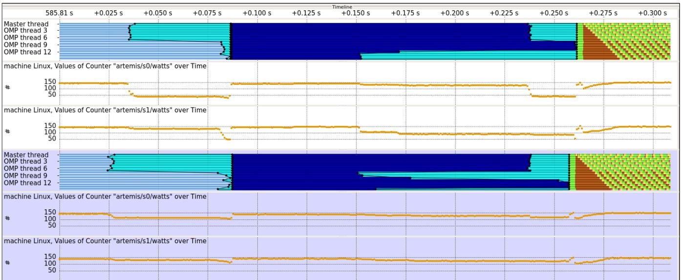
Fig. 8. Screenshot of Vampir comparing a section of two identical runs of SPEC OMP 371.applu on *system B* with different settings for KMP\_BLOCKTIME (white background: set to zero; blue background: default) showing the timeline of the 16 threads each and the power measurements for sockets 0 and 1. OpenMP regions from left to right: parallel `for` (light blue), implicit barrier (cyan), parallel `for` (dark blue), implicit barrier, parallel region (green), barrier (brown).
