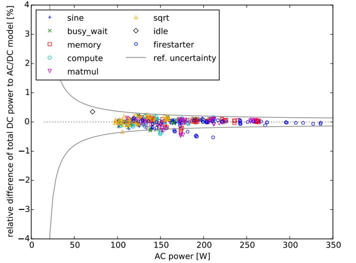
Fig. 7. Relative difference of the total DC shunt measurements compared to a PSU model of the AC reference measurement on *system B*. Includes the uncertainty bound of the reference measurement.
