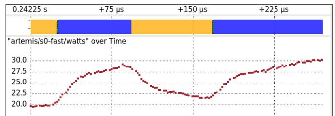
(b) 70  $\mu\text{s}$  load changes and the socket power consumption on *system B*
