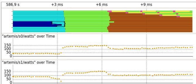
Fig. 9. Screenshot of Vampir of a section of the SPEC OMP 371.applu benchmark detailing the spike in power consumption at +0.260 s in Figure 8.
