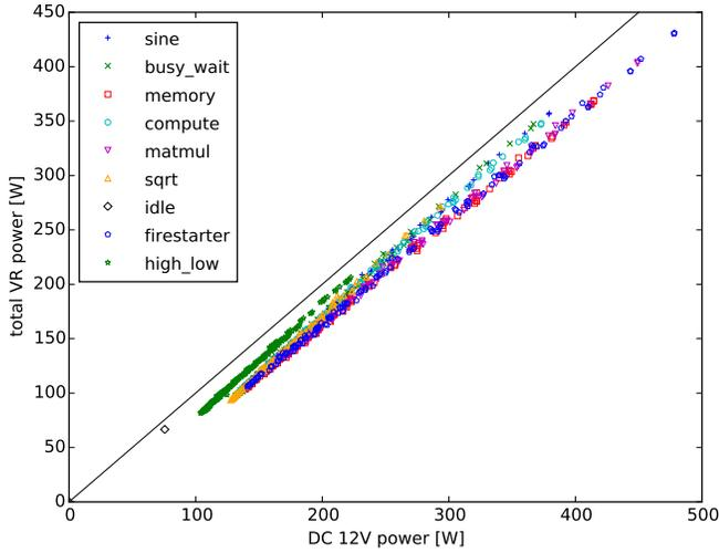
Fig. 3. Measurement points of the 12 V board input measurement compared to the sum of all voltage regulator measurements on *system A* under different load characteristics.
