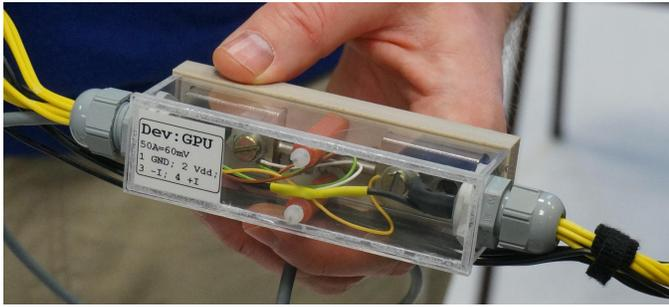
Fig. 2. Measurement shunt inside adapter for 6-pin Molex power connector
