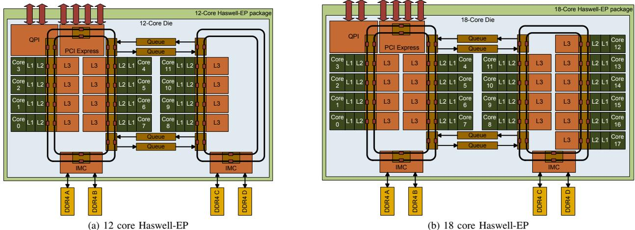
Fig. 1. Haswell-EP implementations with partitioned ring interconnect [6]. The 12-core die (left) is used for 10-core and 12-core units. The 18-core die (right) is used for 14, 16, and 18-core units.
