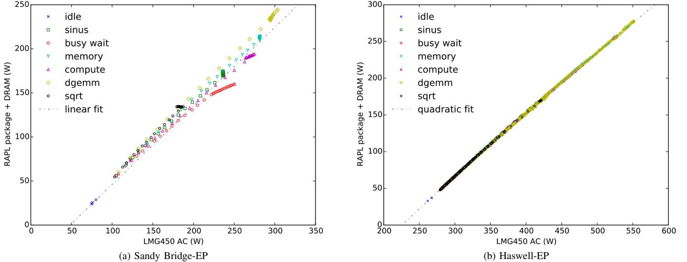
Fig. 2. Comparison of power measurements with RAPL (package + DRAM, sum of two sockets) on Sandy-Bridge EP [20] and Haswell-EP versus total system power consumption (AC) measured with a high-accuracy power meter. Note that the different x-axis ranges are due to the full speed fan settings on the Haswell-EP system which does not affect RAPL accuracy.
