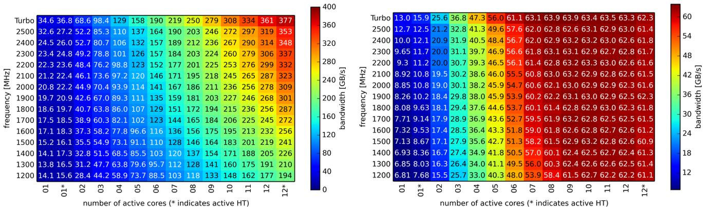
Fig. 8. Read bandwidths from Level 3 cache (left) and DRAM (right) depending on concurrency and frequency
