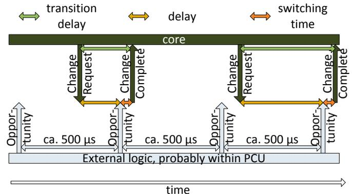
Fig. 4. Presumed mechanism for p-state changes on Intel Haswell-EP processors.
