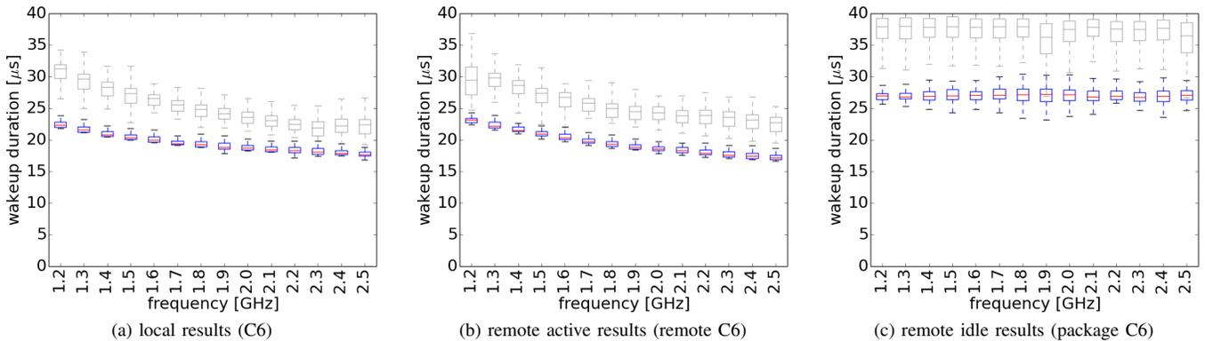
Fig. 6. Idle transition latencies for different C6 scenarios in comparison to Sandy Bridge EP processors (grey)
