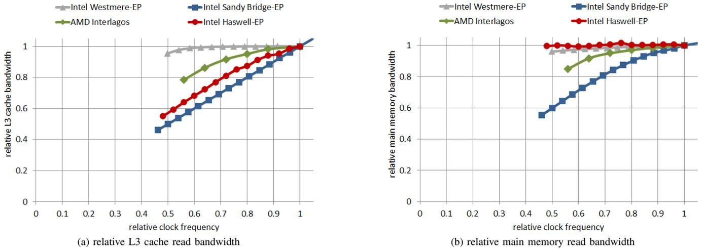
Fig. 7. Scaling of shared main memory and L3 cache bandwidth at maximum thread concurrency, normalized to the bandwidth at base frequency.
