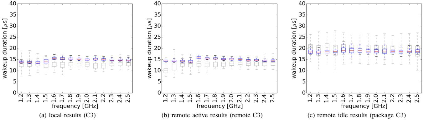
Fig. 5. Idle transition latencies for different C3 scenarios in comparison to Sandy Bridge EP processors (grey)
